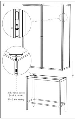
2. Connect the base and cabinet in all four corners using the 16mm screws and 5mm hex key. Place the two shelves inside the cabinet. Place the cabinet onto the base.
