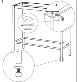
3. Use the adjustable feet to level the Haze Vitrine. Check if the Vitrine is level using a spirit level. Mount the doors onto the cabinet.
