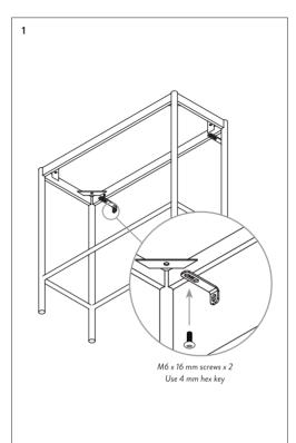
1. Place the base of the Haze Vitrine against the wall. Mount the wall safety sets onto the base. Do not fully tighten the screws yet.
